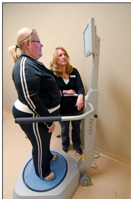
The Biodex Balance System is a computerized instrument that measures a patient’s static and dynamic vestibular balance and proprioception. It enables objective, graphic demonstration of the vulnerability of patients to a fall vs. age-matched normal, and provides a series of assessment challenges, presents patient performance in real time on a large heads-up computer screen. It stores that performance for retrieval, progress assessment and printout for medical records.
